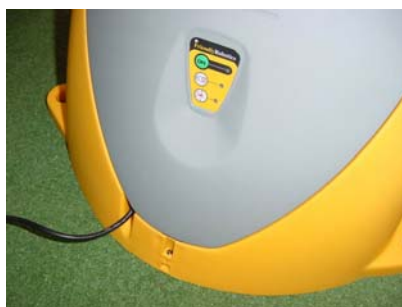
Figure 1.21 – Proper position of the Power Supply cable
