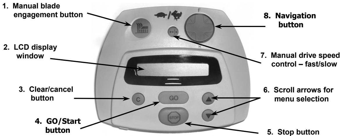
Figure 2.3 - Manual Controller Layout
