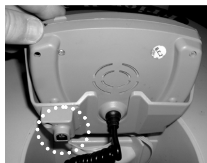
Standard charger connector socket
