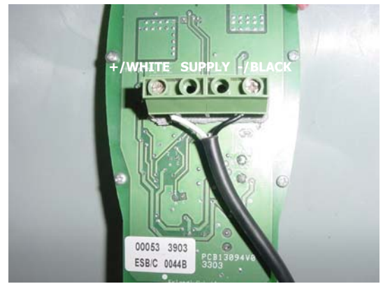
Figure 1.19 Power Supply Cord Track through the cover
