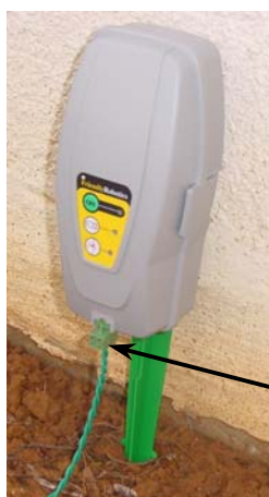
Figure 1.34 – Perimeter Switch with mounting stake attached
