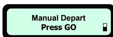
Figure 5.2 – LCD Display on Robomow when docked and NO Weekly Program is set OR the 'Auto Depart' function is turned off
