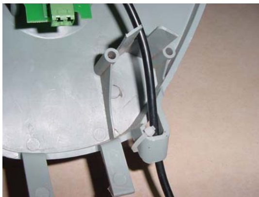
Figure 1.18 Routing the Power Supply cord into the cover
