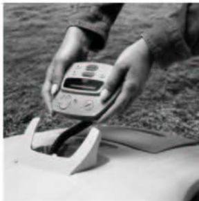
Figure 3.9 - Removing the Manual Controller from its' holder
